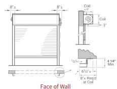
Maintains clearance of full opening, minimal exposed components.
